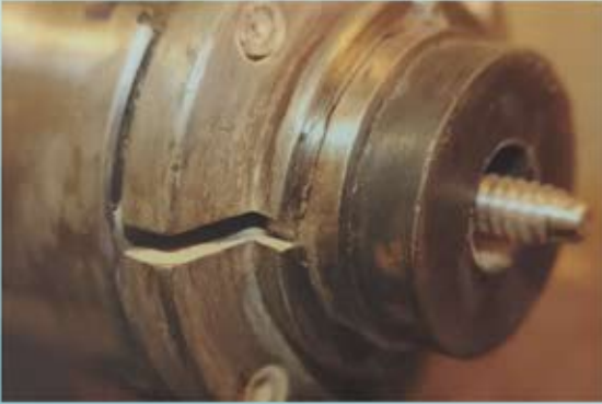
Ring magnet attached to a standard screw chuck
